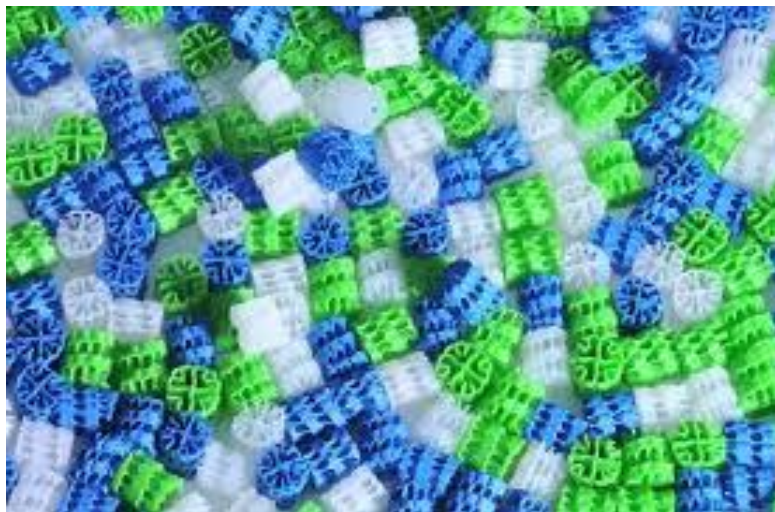
Figure 2: Polyethylene carrier element of MBBR (Source: lenntech.com/processes/mbbr.htm)
