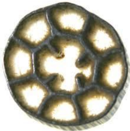
Figure 3: Biofilm in polyethylene carrier element (Source: lenntech.com/processes/mbr.htm)
