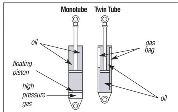
Figure 4.2: Types of Shock absorber
