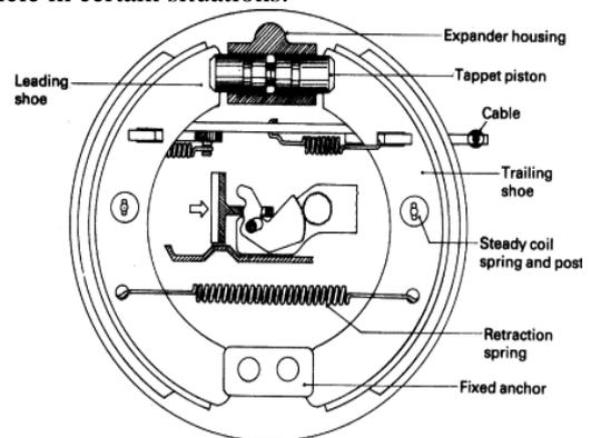
Figure 3.6: Braking System
