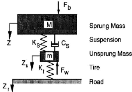
Figure 6.1: Quarter Vehicle Suspension Model
