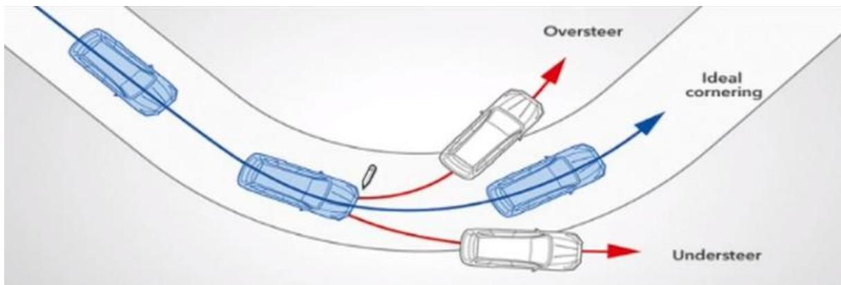
Figure 7: Unpredictable Steering
