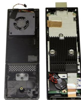
Figure 1: Inside view of Intel Compute Stick
