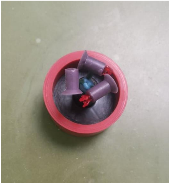
Figure 2: Wax patterns of the test samples of BioHPP.
