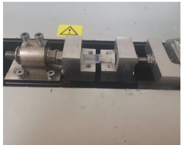
Figure 5: The grips mounted on the testing machine
