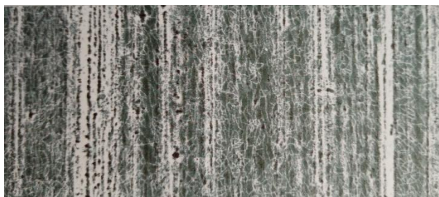
Figure 3.3 A: Scanning Electron Micrograph at 20 kV of standard conversion coating
