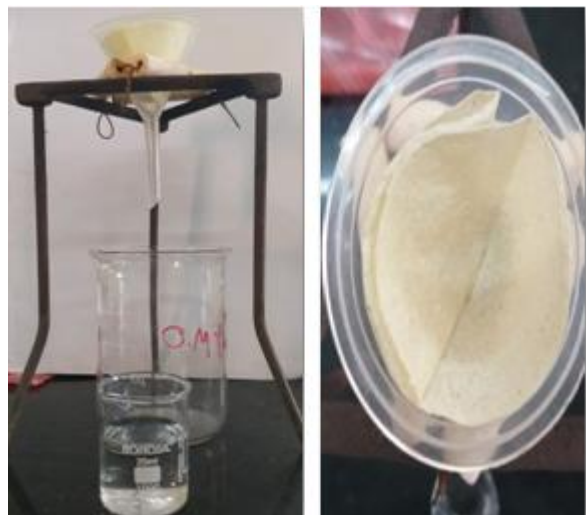
Figure 9: Testing the Water retention Capacity.
