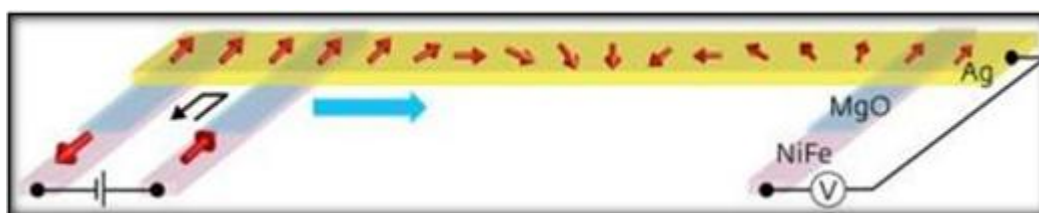
Figure 10: Setup to measure spin signal into a thin silver wire
