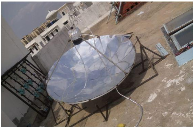
Figure 2: Parabolic Dish Type Solar Concentrator
