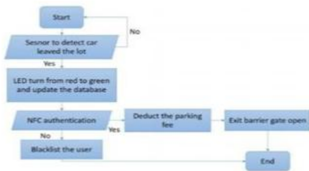
Figure 10: Flow chart of NFC Working (2)
