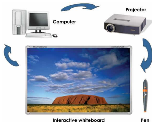
Figure 1: Parts that make up the digital interactive board system
