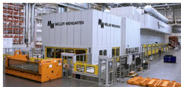
Figure 2 .High volume “Compact” Automotive cross bar press (Schuler Automation)
