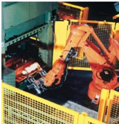
Figure 4 (a and b) Standard 6 axis Robot model IRB 7600for handling crankshaft for Auto-Industry [12]
