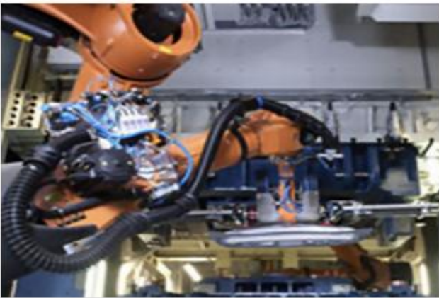
Figure 3: “Crossbar Robot” transfers part directly from press to (Scheler Automation)
