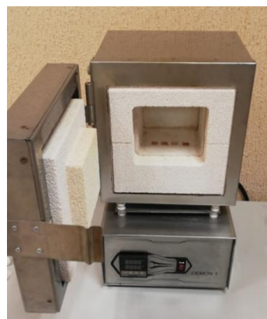
Figure 3: Image of the muffle furnace and copper sheets used in the standardized process of thermal oxidation of copper
