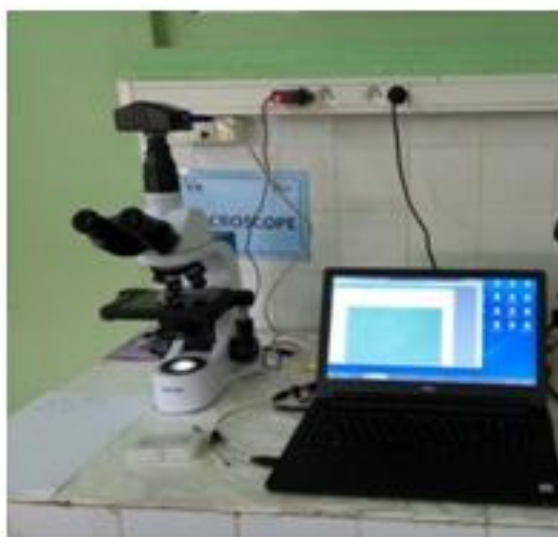
Device for particle size distribution by microscopy and calibration of the particle size slide
