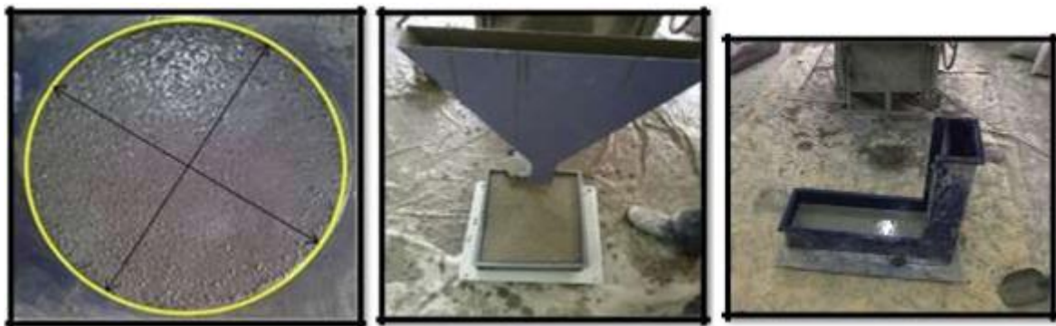
(a) Slump Flow Test (b) V-funnel flow time test (c) L-box test
