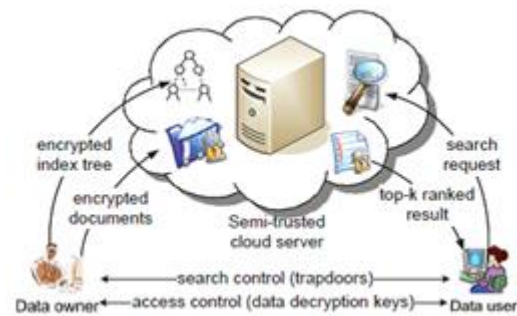
Figure 1: The architecture of ranked search over encrypted cloud data
