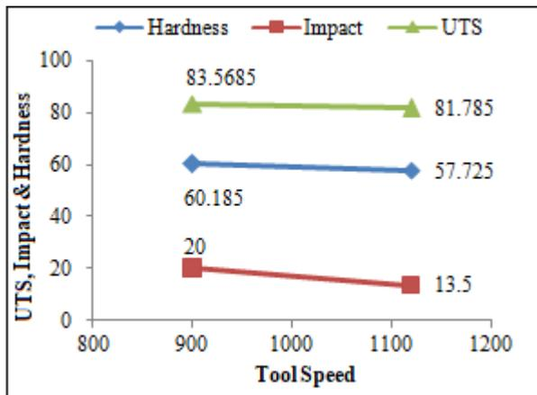
Graph 1: Tool Speed vs Ultimate stress, Impact Strength & Hardness
