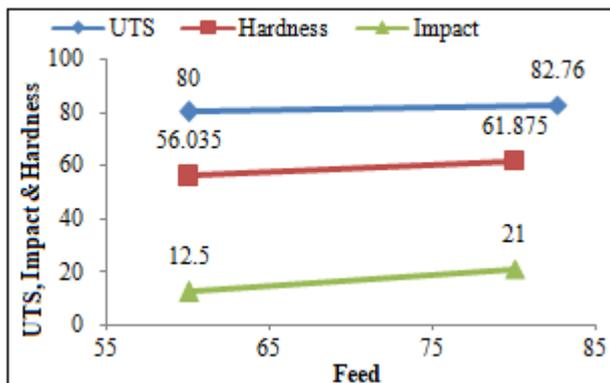
Graph 2: Tool Feed vs Ultimate stress, Impact Strength & Hardness
