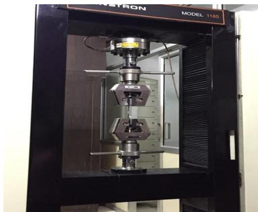
Figure 5: Specimen mounted over the universal testing machine (Instron)
