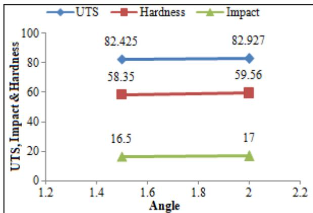
Graph 3: Tool Angle vs Ultimate stress, Impact Strength & Hardness
