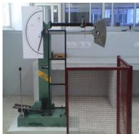
Figure 7: Impact testing machine
