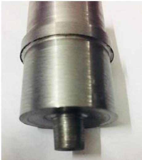
**Figure 2:** FSW Tool used in the present work
