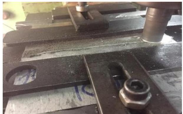
Figure 1: Friction stir welding Process
