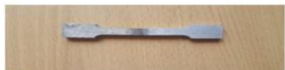
**Figure 4:** Image showing the sample of tensile test specimen
