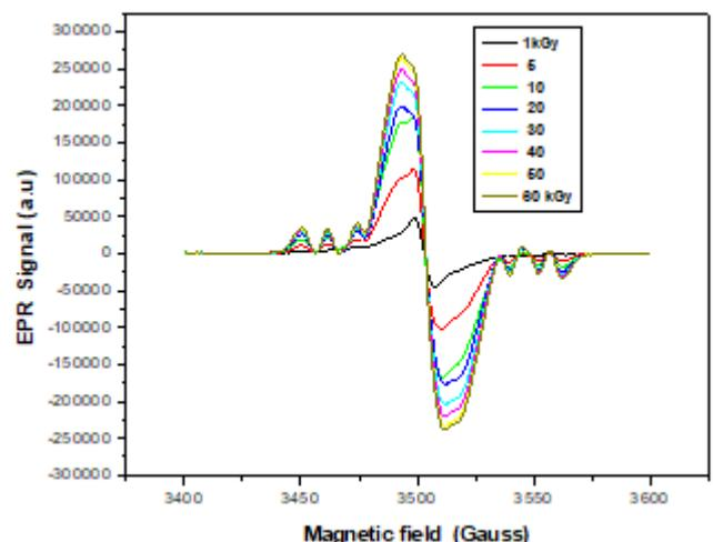
**Figure 2:** Amplitude of the EPR Signal as a function of high doses
