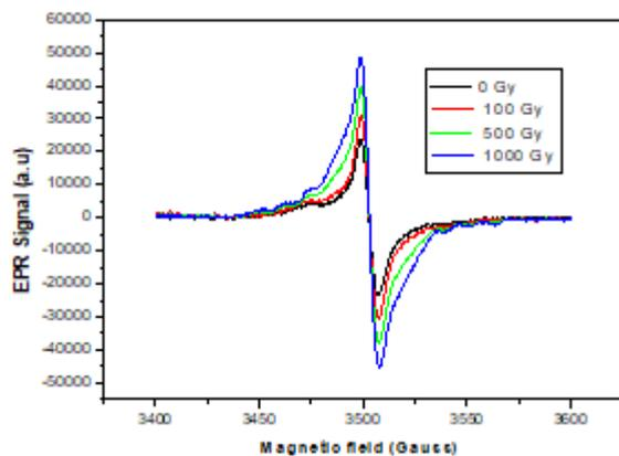
**Figure 2:** Amplitude of the EPR Signal as a function of low doses
