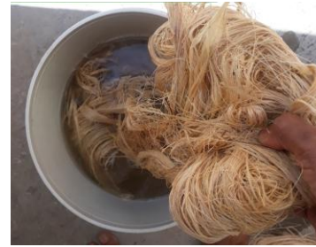
Figure 2: Sisal fiber in NaOH solutions
