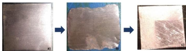
Figure 3: a) Cu foil with size of 20 mm × 20 mm and 300 μm of thickness. b) Cu foil of 100 μm in thickness after thinning. c) Cu foil of 100 μm in thickness dimensioned at 5mm × 5mm.
