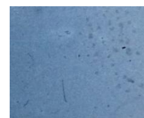
Figure 4: Zn film obtained by thermal evaporation
