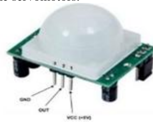
Figure 5: Passive InfraRed sensor for motion detection
