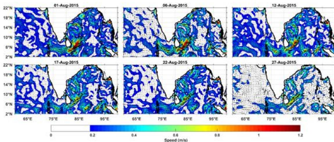
**Figure 3:** Surface currents during August 2015 from OSCAR data. Arrows represents the flow direction and color represents the magnitude of the speed (m/s). Current speed between 0 – 0.2 m/s is set to white for the clear identification of water exchange between AS and BoB
