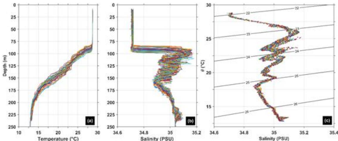
**Figure 6:** Temperature and Salinity characteristics (a) temperature profiles, (b) salinity profiles, and (c) T-S diagram estimated from *RV Roger Revelle* CTD data (48 casts) during 11 August 2015 at  $6.42^\circ$  N,  $85.21^\circ$  E. Color represents the individual CTD profiles. Measurements were taken from surface to a depth of 250 m
