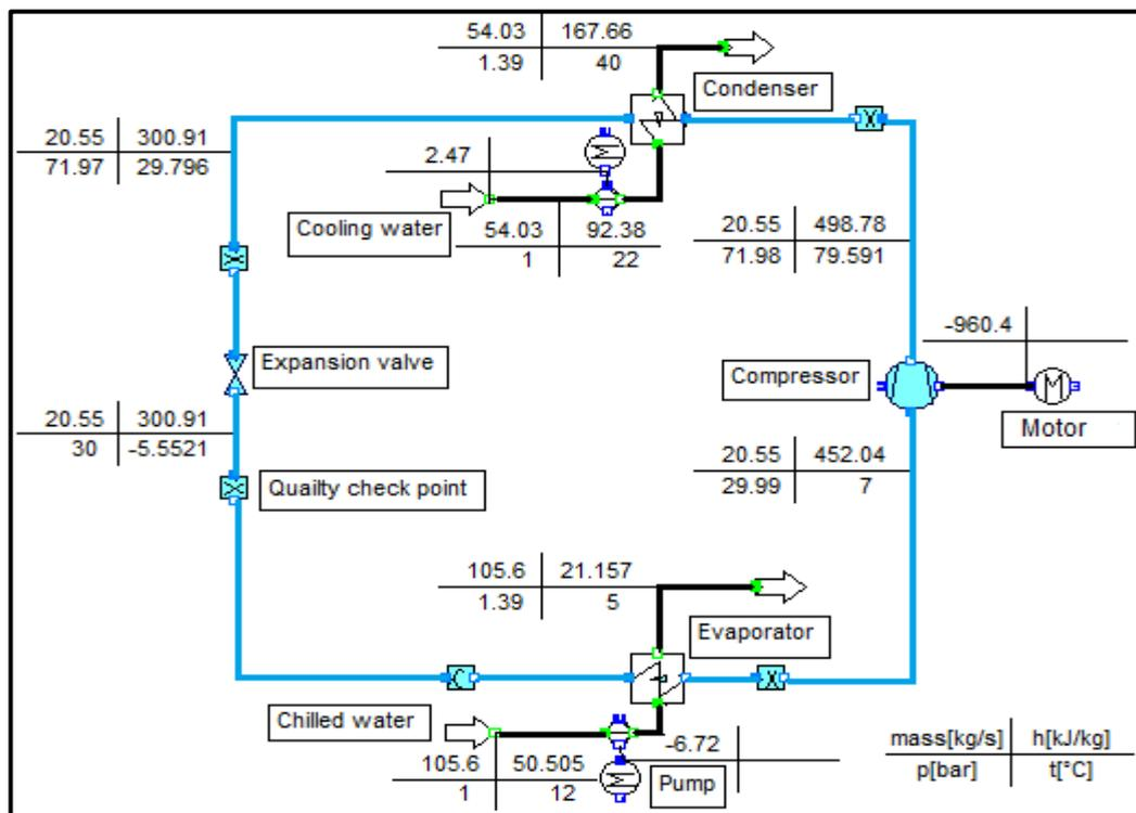
Figure 3: Refrigeration capacity produced by R-744 vapor compression cycle model
