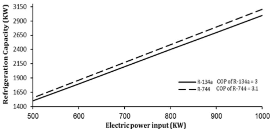
Figure 5: Effects of the electric power input variations on the refrigeration capacity
