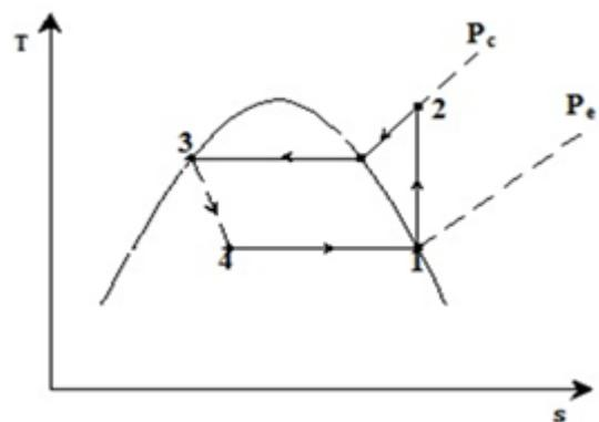
**Figure 2:** Basic vapor compression refrigeration cycle T-s diagram
