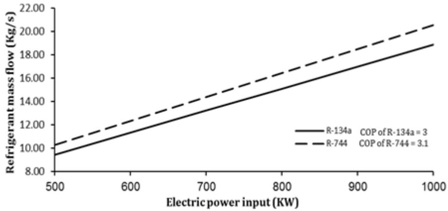
Figure 6: Effects of the electric power input variations on refrigerant mass flow
