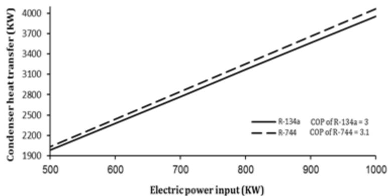
Figure 9: Effects of the electric power input variations on condenser heat transfer
