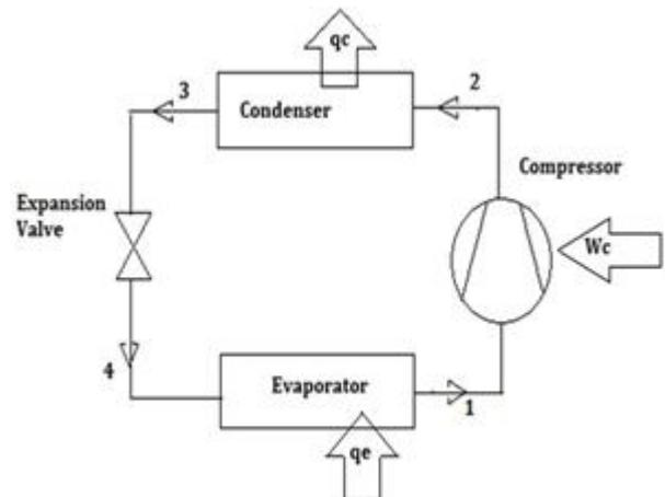
**Figure 1:** Basic vapor compression refrigeration cycle
