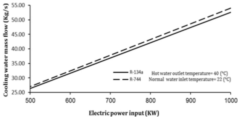
Figure 8: Effects of the electric power input variations on cooling water mass flow
