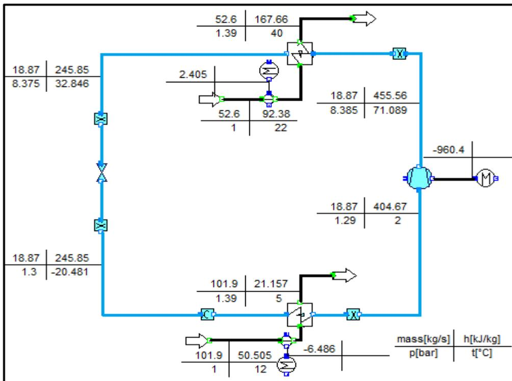
Figure 4: Refrigeration capacity produced by R-134a vapor compression cycle model
