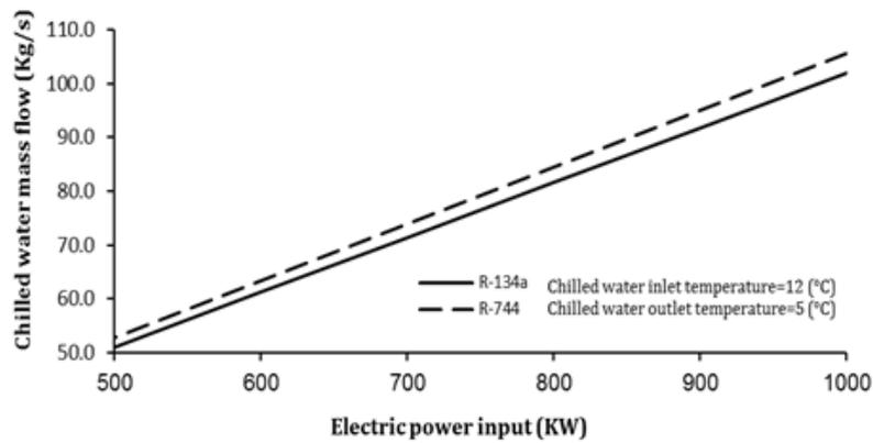
Figure 7: Effects of the electric power input variations on the chilled water mass flow
