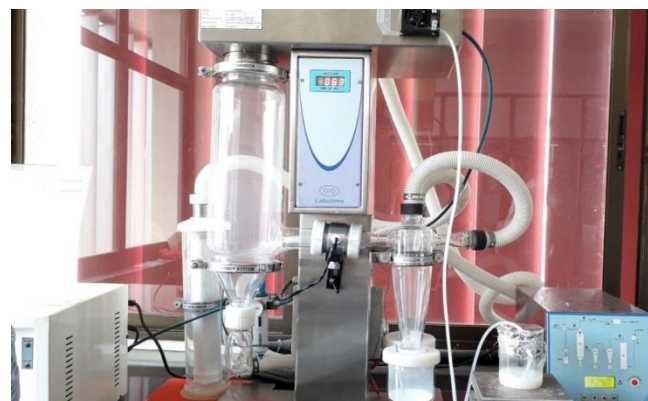
Figure 2: Preparation of Solid SLN by spray Drier
