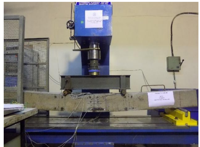
Figure 3: Concrete crushing at top at ultimate load
