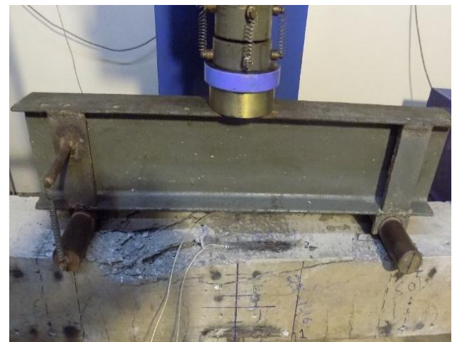
Figure 4: Close-up view of concrete crushing at top of the beam at ultimate load
