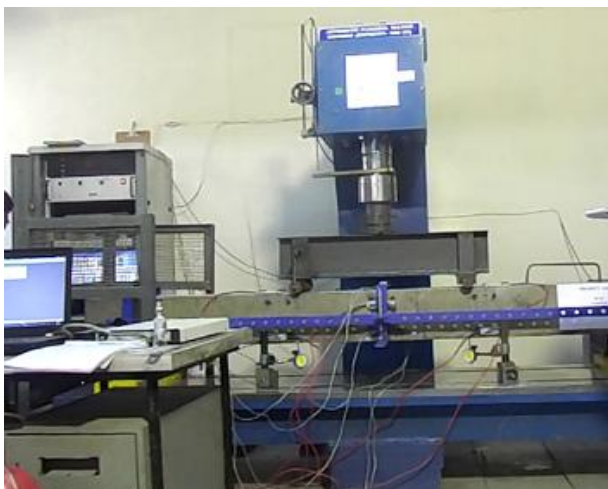
Figure-1: Test set up for Flexural Strength of Reinforced Concrete Beams
