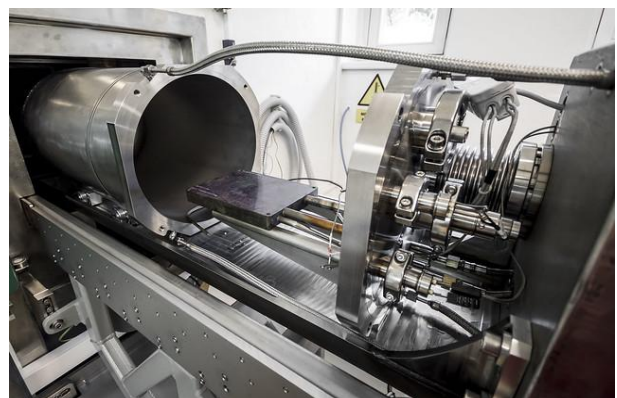
Figure 1: Experimental irradiation box with heating cassette/sample holder.
