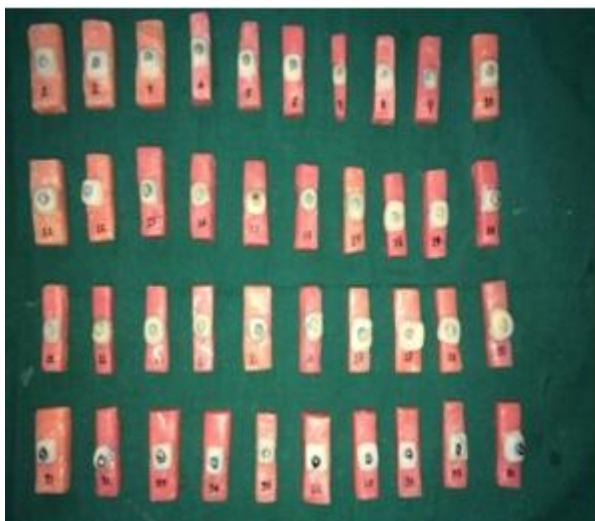
Figure 5: Group 1- metal screw posts, Group 2- glass fibre posts, Group- carbon fibre posts, Group 4- cast metal posts (each group contains 10 samples ) Figure:6. Fractured samples
