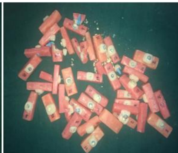
Figure 5: Group 1- metal screw posts, Group 2- glass fibre posts, Group- carbon fibre posts, Group 4- cast metal posts (each group contains 10 samples ) Figure:6. Fractured samples
