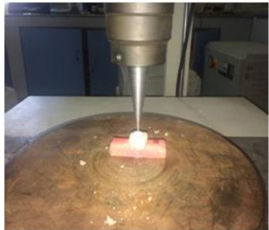
Figure 4: Fracture of tooth samples under universal testing machine at 90° at the cross head speed of 1 mm per minute
