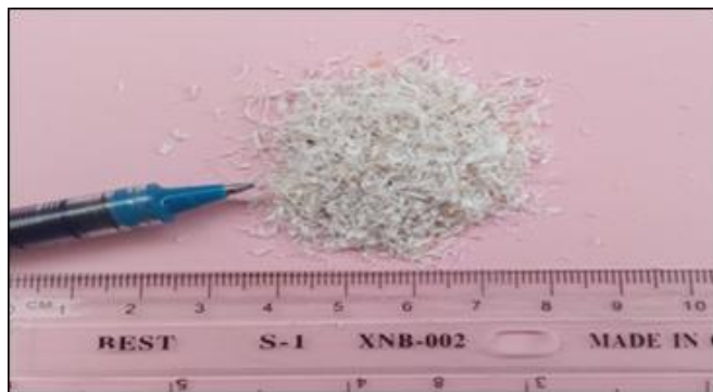
Plate 1: locally waste PVC used in this study
