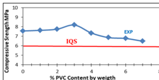
Figure 2: A comparison between IQS and waste PVC used in study on compressive strength
