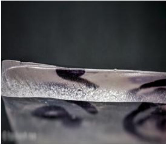
Figure 6: Macro Photograph (1:1) of unreinforced fractured PMMA specimen showing micro-cracks
