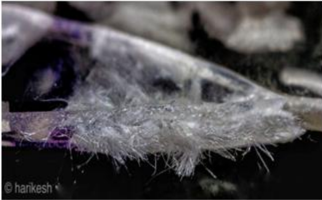
Figure 13: Macro photograph (1:1) of fractured specimen of Nylon Fibers showing the structure of the fiber that is soft and irregular
