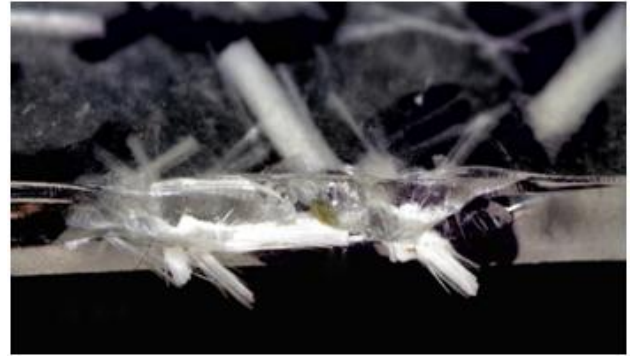
Figure 9: Macro photograph (1:1) of Glass Fibers showing the projection of fibers from the fractured surface
