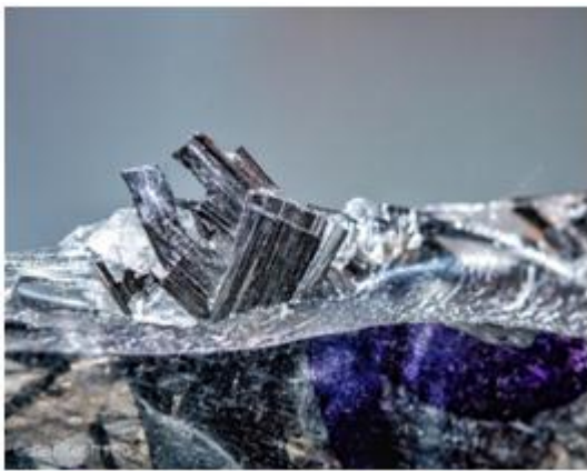
Figure 7: Macro photograph (1:1) of fractured specimen of Carbon Fibers showing improper bonding of the fibers with the resin matrix
