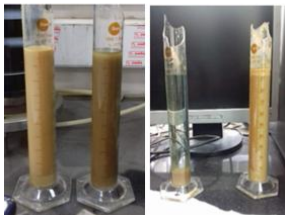
Figure 5: Free Swell Index Test
