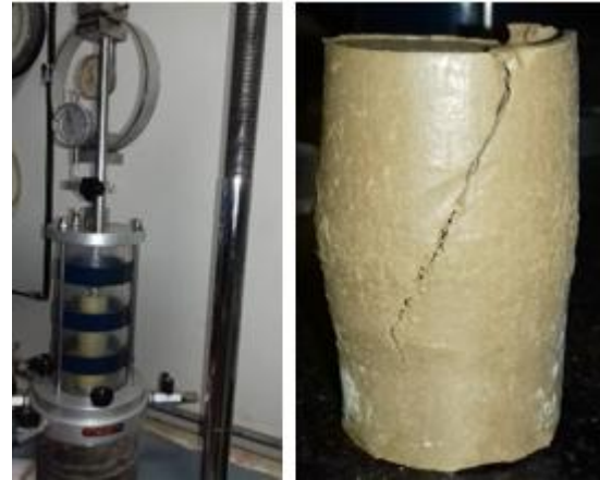
Figure 8: UCS Test (a) Triaxial Loading Apparatus (b) Specimen
