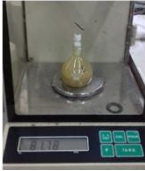
Figure 6: Determination of Specific Gravity
