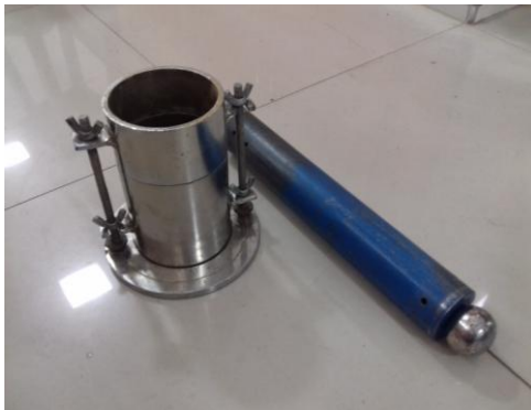
Figure 7: Standard Proctor mould and rammer
