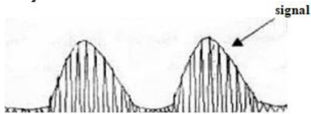
Figure: Rectified muscle contraction signal
