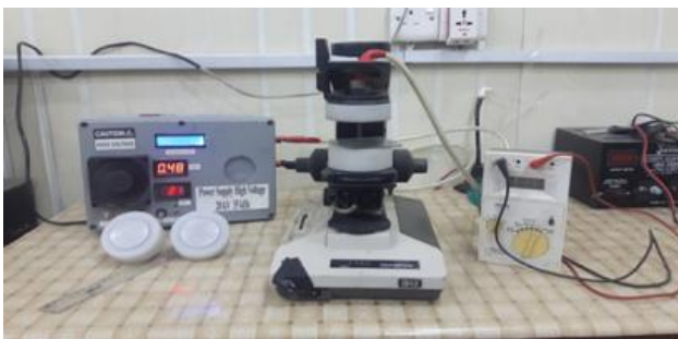
Figure 2: The locally designed DBD Plasma system.
