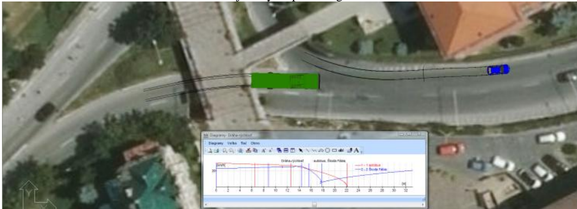
Figure 5: View of the bus and car movement with a trajectory – speed diagram
