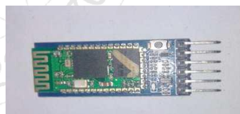
Figure 5: Bluetooth Module (HC-05)
