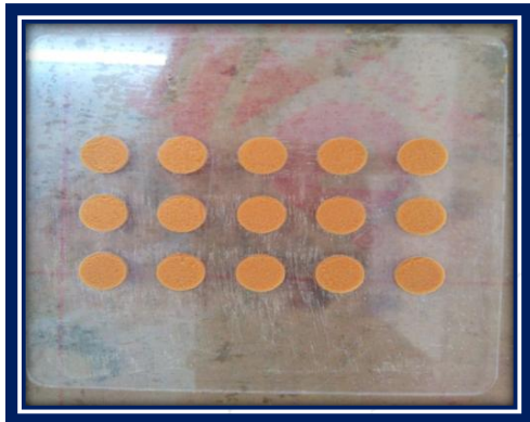
Figure 2: Sample discs prepared in a mold of 10mm in diameter by 2mm in thickness.
