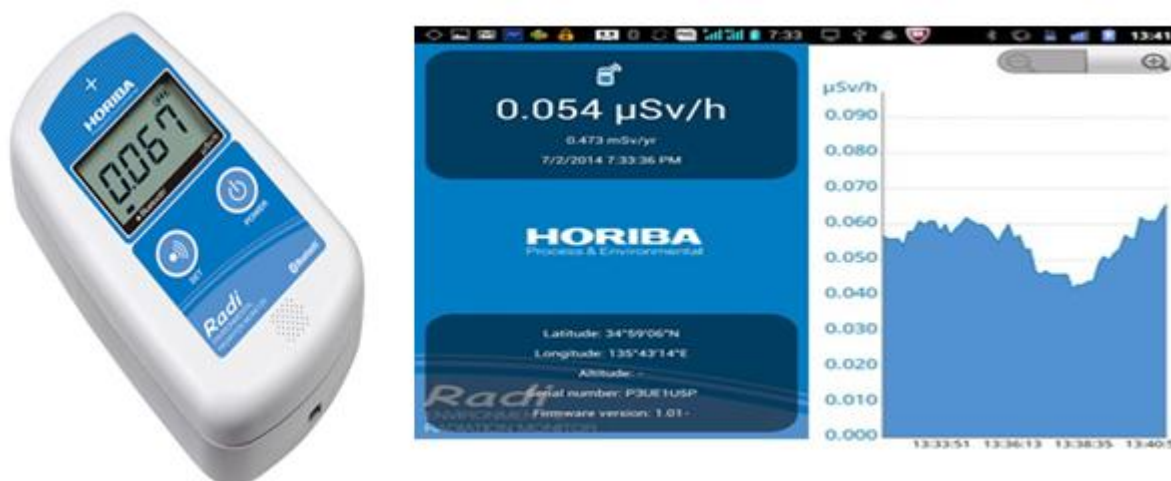
Figure 3: View of Environmental radiation monitor PA-1100 Radi
