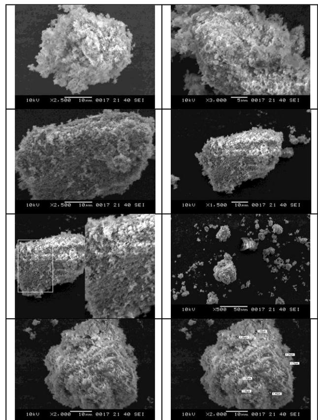
Plate 9: Scanning electron microscopy images of clay sample showing their morphology and particle size
