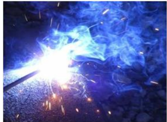
Figure 3: Shielded Metal Arc Welding
