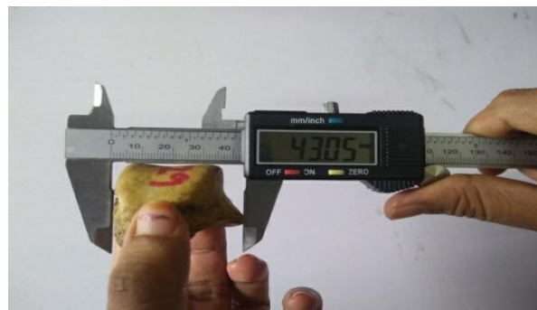
Figure 2: Showing the method of measurement of Maximum transverse width
