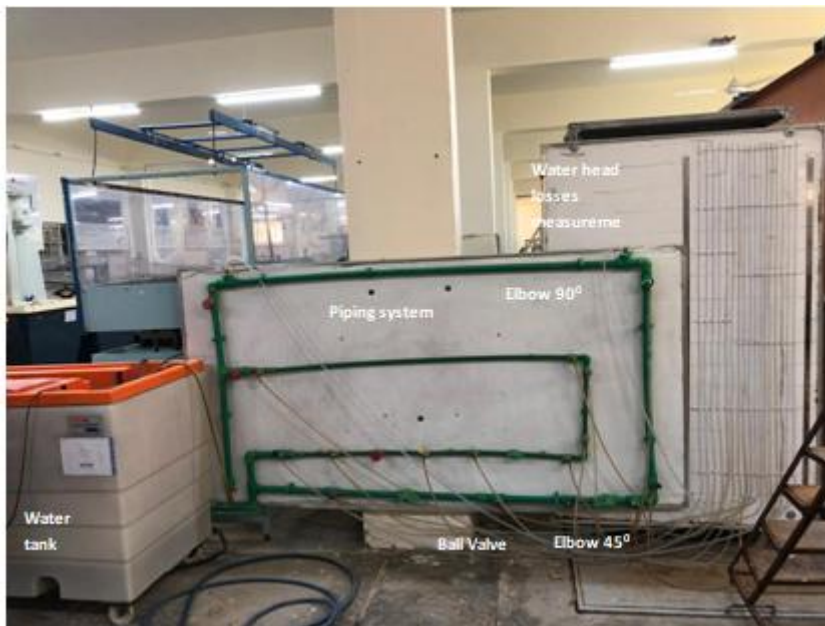
Figure 1: Piping system used
