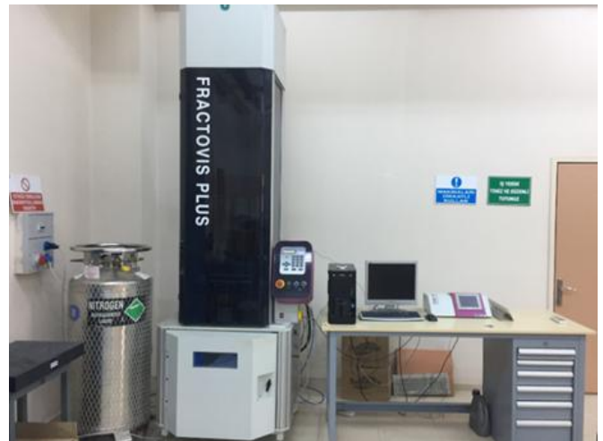
Figure 2: CEAST 9350 (Fractovis Plus) impact tester
