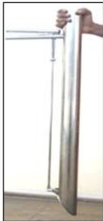
Hand lever operated stainless steel trans-planter (90 cm height and 1.76 kg weight)
