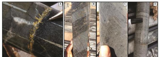
Figure 4: Samples of Visible Gold (A) and Disseminated (B) and Non-Mineralized (C), Mineralized Granitoid (D)
