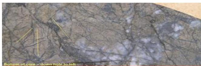
**Figure 3:** Hydrothermalized, brecciated and highly mineralized basalt sample
