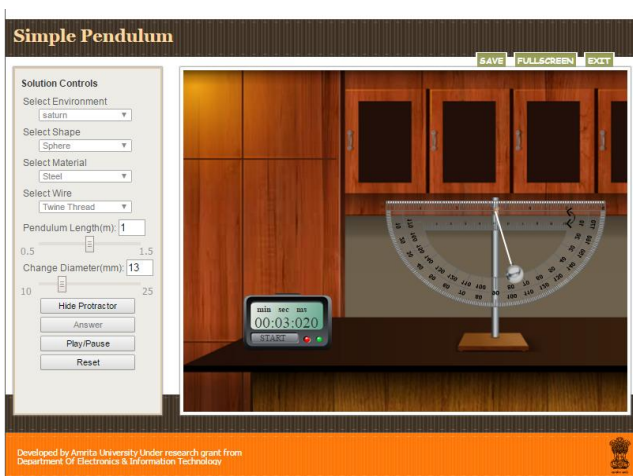
Figure 3.2: Illustration of the use of a simple pendulum To plot a L-T 2 graph
