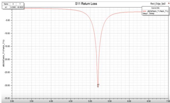
Figure 5: Return loss using HFSS
