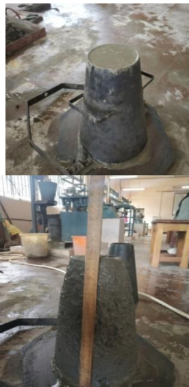
Figure 4: Slump test set up
