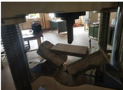
Figure 7: Shows the test setup of modulus of rupture
