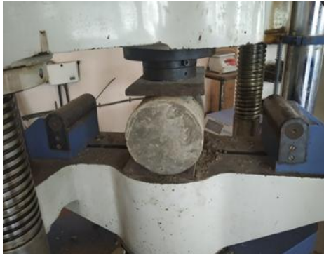
Figure 6: Split tensile test
