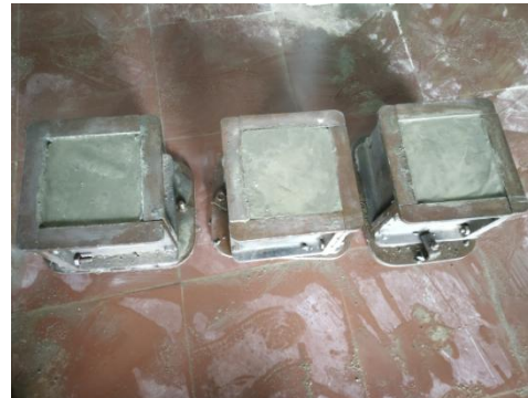
Figure 5: Casting of cubes
