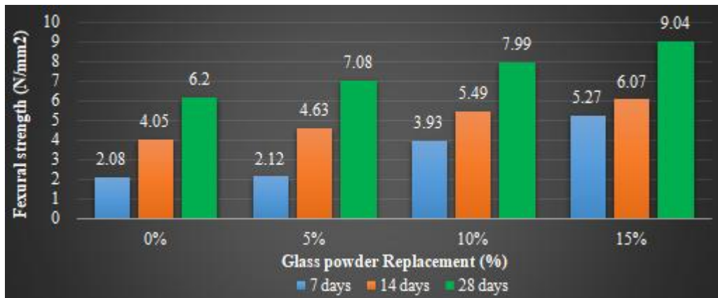
Figure 2: Comparative flexural strength of various percentage replacement of glass powder with cement
