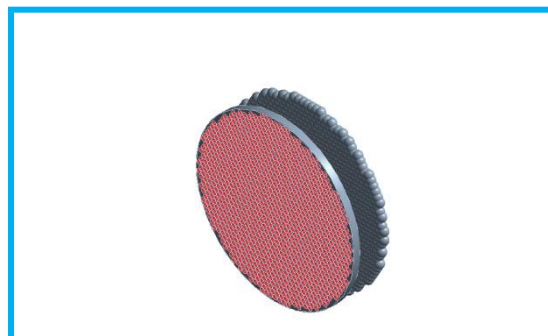
Figure 13: Point mass of 2.5 kg of each tube at its C.G.
