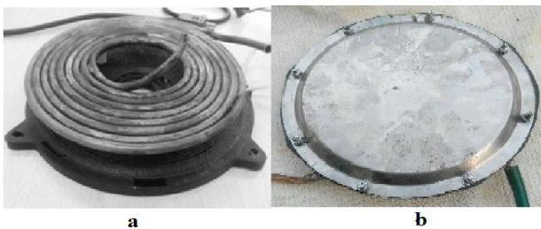
Figure 3: Construction of Load Coils a) MS load coil b) SS load coil
