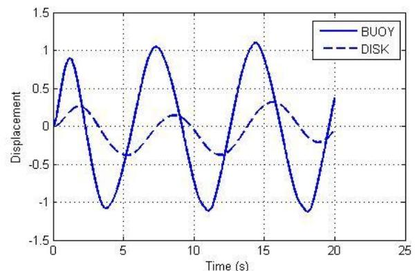
Figure 2: Displacement of BUOY and DISK with the function of harmonic wave:  $x(t) = \cos(2\pi f t + \varphi)$ , with  $f = 1 / 7$ ,  $\varphi = \pi$ .
