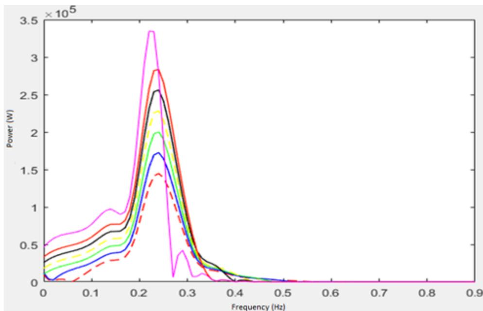
Figure 11: Mean power adsorbed for each wave frequency
