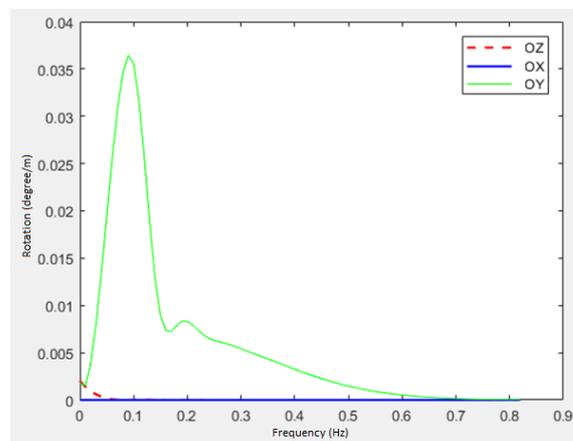
Figure 8: Amplitude of rotation – RAOs for buoy 1
