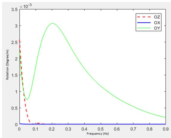
Figure 10: Amplitude of rotation - RAOs for buoy 2
