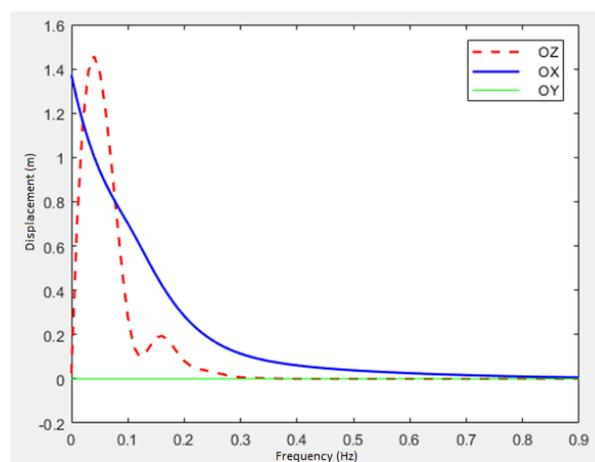
Figure 9: Amplitude of translation – RAOs for buoy 2
