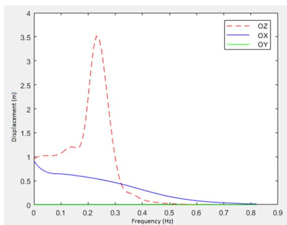
Figure 7: Amplitude of translation – RAOs for buoy 1
