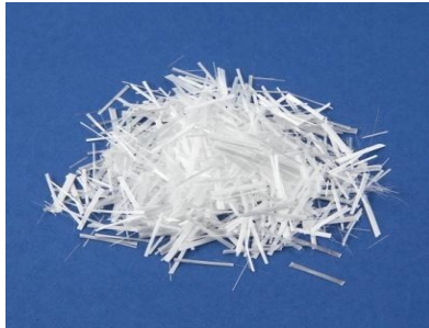
Figure 3: Glass Fibre (Length = 36 mm), (as per IRC: 15 – 2011)
