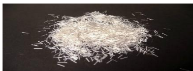
Figure 1: Glass Fibre (Length 36 mm –as per IRC 15 – 2011)
